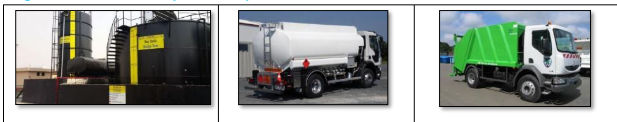
Figure 3: MARPOL compliant receptacles
